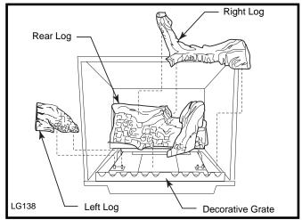
Fig. 43 Install back, right and left logs.
